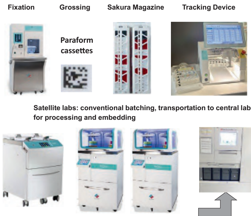
Fig. 3 ▲ Formalin fixation of tissue samples in the operating tract using the Ultrasafe (Milestone, Bergamo, Italy) dispensing unit, grossing, assembly of cassettes in magazines, and tracking prior to transportation and further processing in tissue processors and a Sakura AutoTEC a120 (Sakura, Alphen aan den Rijn, NL) embedding unit
