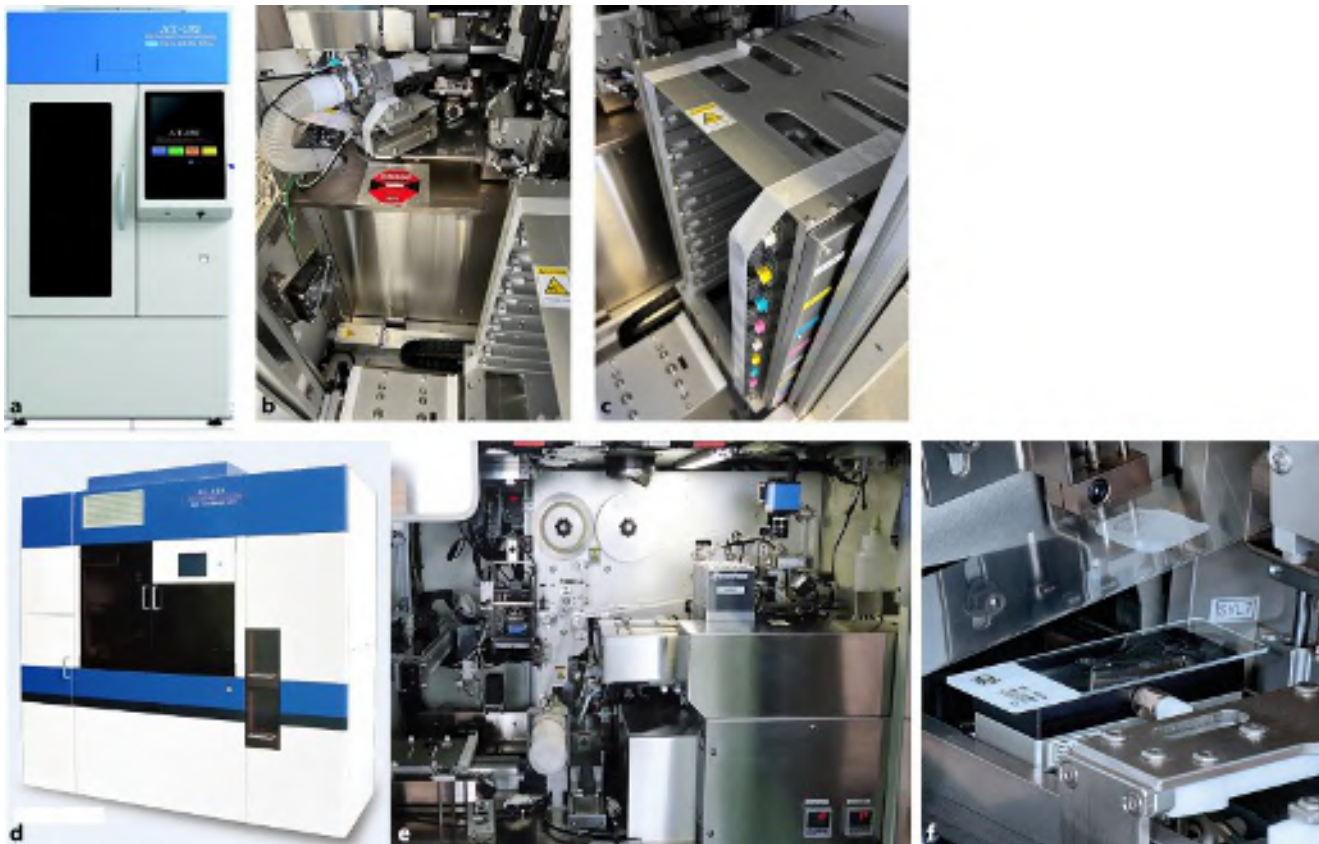
Fig. 2 ▲ Automatic microtomes AT-192 and AS-410M (Dainippon Seiki). a The AT-192 facing microtome handles up to 192 paraffin blocks; b,c view into the microtoming chamber with a reservoir for 8 \times 24 blocks. d The AS-410M instrument; e view inside the microtoming unit, the transfer tape, and transfer of a section to a glass slide with dedicated printed label ( f )
