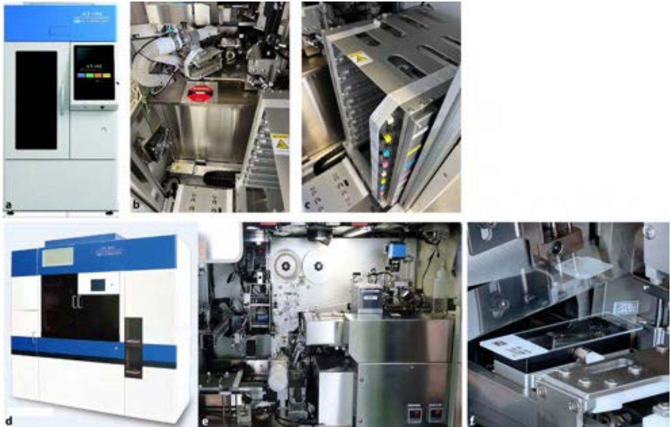
Fig. 2 ▲ Automatic microtomes AT-192 and AS-410M (Dainippon Seiki). a The AT-192 facing microtome handles up to 192 paraffin blocks; b, c view into the microtoming chamber with a reservoir for 8 × 24 blocks. d The AS-410M instrument; e view inside the microtoming unit, the transfer tape, and transfer of a section to a glass slide with dedicated printed label ( f )
