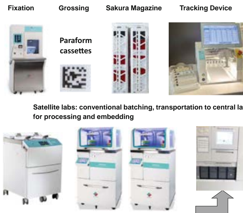
Fig. 3 ▲ Formalin fixation of tissue samples in the operating tract using the Ultrasafe (Milestone, Bergamo, Italy) dispensing unit, grossing, assembly of cassettes in magazines, and tracking prior to transportation und further processing in tissue processors and a Sakura AutoTEC a120 (Sakura, Alphen aan den Rijn, NL) embedding unit
