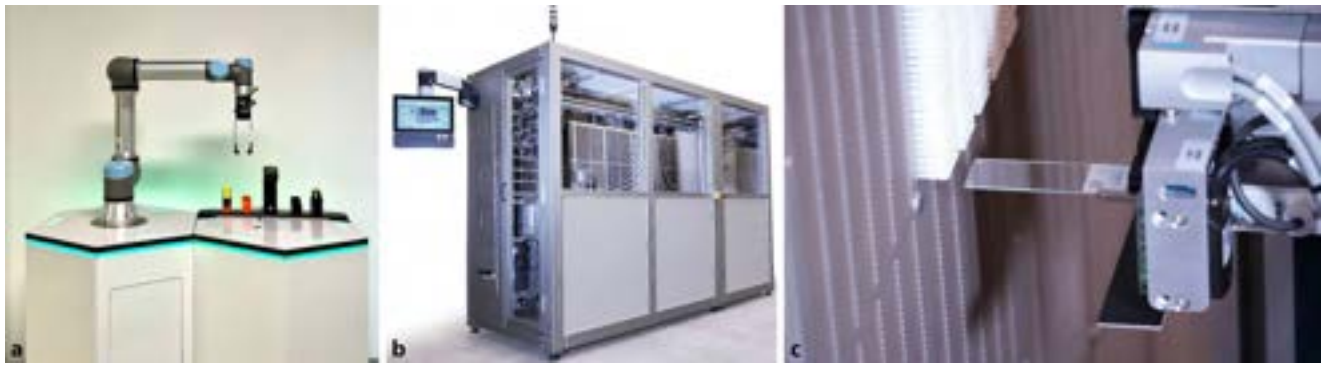
Fig. 4 ▲ Slide handling using collaborative robot UR5e (a) and short- to medium-term storage of 2D-coded slides in the Axlabs Slidemanager (b, c)
